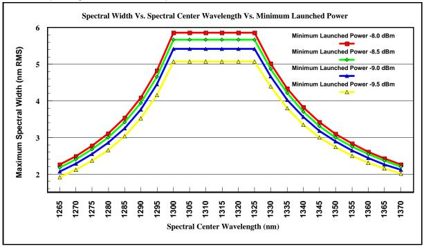
Figure 2 – 100-SM-LC-L transmitter specifications
